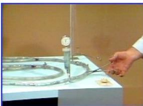
However, there may be other factors that can reduce flow, even in the presence of a positive mean vascular pressure. The most obvious candidate is resistance. Certainly a tube clamp placed partially across a vessel will add considerable resistance to flow. Let's see what effect such resistance does have on pump output.
